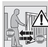
All persons using the gate system must be shown how to operate it properly and safely. Demonstrate and test the mechanical release as well as the safety return. To do this, halt the closing gate by grasping it with both hands. The gate system must initiate the safety return.
